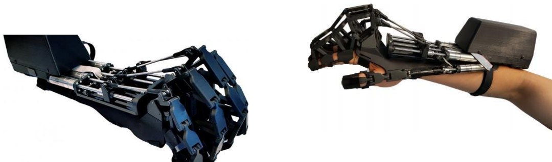
Figura 2 – Exoesqueleto bilateral ( Bilateral hand exoskeleton for stroke rehabilitation ) desenvolvido na University of Technology Sydey (UTS). Fonte: UTS site.
