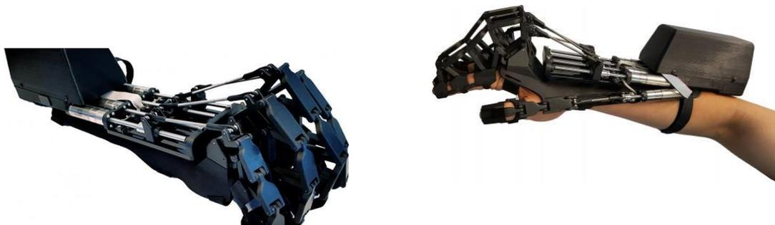
**Figura 2** – Exoesqueleto bilateral (*Bilateral hand exoskeleton for stroke rehabilitation*) desenvolvido na University of Technology Sydney (UTS). Fonte: UTS site.
