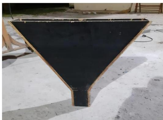
**Figura 7-** Funil - V fabricado. **Fonte:** Autor
