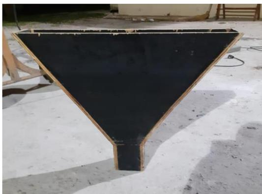
**Figura 7-** Funil - V fabricado. **Fonte:** Autor
